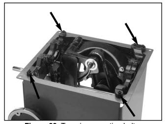
Figure 28. Trunnion mounting bolts.
